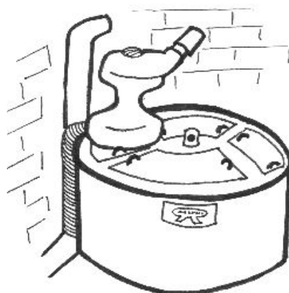
Fig. 7.13 – Aquatron faecal separator. Pipe from toilet at upper right; pipe from grey water fittings at upper left. Image: Susie Harty
