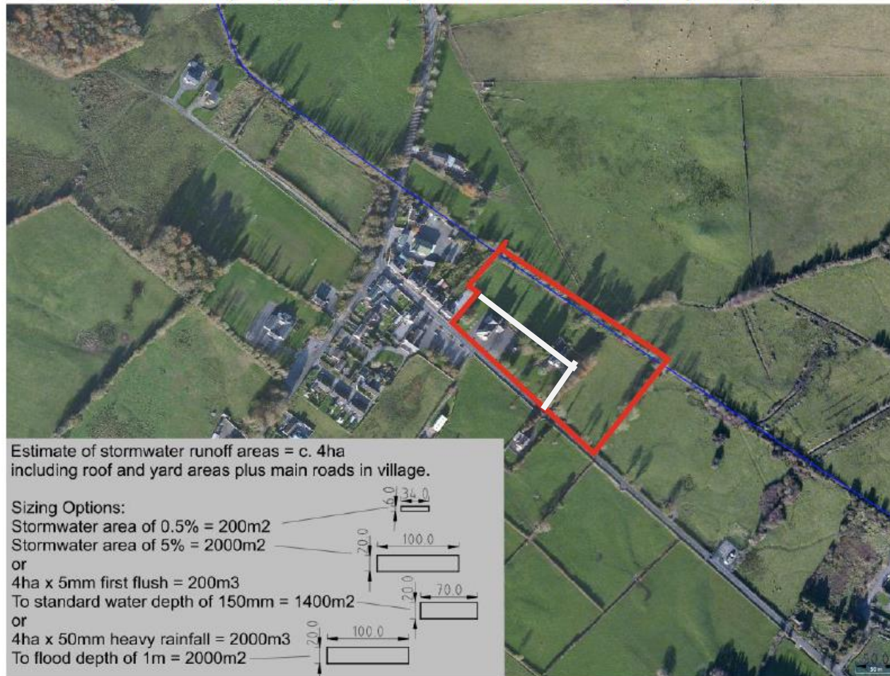
Fig. 10.1 – Examples of sizing options for a stormwater wetland for the full village
